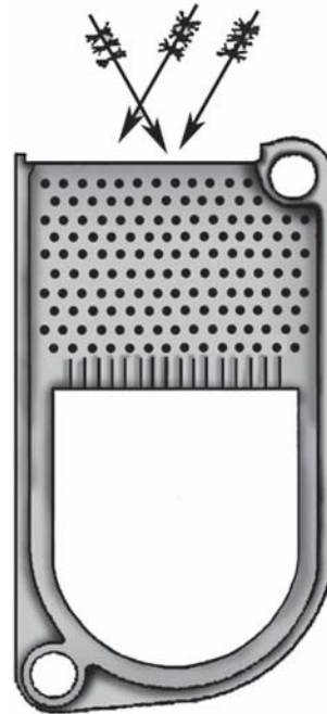
Figure 15 - Brush Diagonally Through Flue Passages
