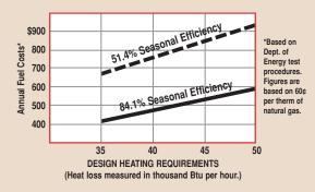
This graph illustrates the difference in annual operating costs between boilers with higher and lower efficiencies. Boilers installed years ago have seasonal efficiencies as low as 50%. So, your savings in fuel dollars with Utica's MGB boiler can repay its installed cost in a few short years!
