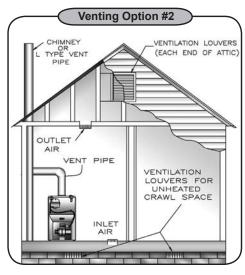
When communicating with the outdoors by means of vertical ducts, each opening shall have a minimum free area 1 square inch per 4,000 Btu per hour of total input rating of all appliances in the enclosed space.
