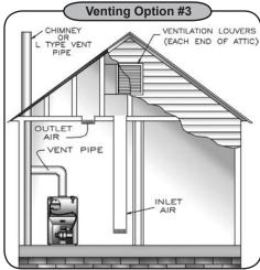
If horizontal ducts are used, each opening and duct shall have a minimum free area 1 square inch per 2,000 Btu per hour of total input rating of all appliances in the enclosed space.
