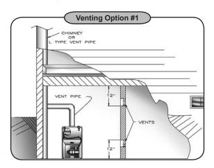
When the boiler is installed in a confined space and all air is provided from the outdoors the confined space shall be provided with one or two permanent openings. When ducts are used, they shall be of the same cross sectional area as the free area of the area of the openings to which they connect. The minimum dimension of rectangular air ducts shall be not less than 3 x 3 inches or 9 square inches. **Venting Option #1**
