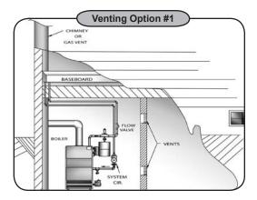
When the boiler is installed in a confined space and all air is provided from the outdoors the confined space shall be provided with one or two permanent openings (See MGB Installation manual for more detailed). When ducts are used, they shall be of the same cross sectional area as the free area of the area of the openings to which they connect. The minimum dimension of rectangular air ducts shall be not less than 3 x 3 inches or 9 square inches. *Venting Option #1*
