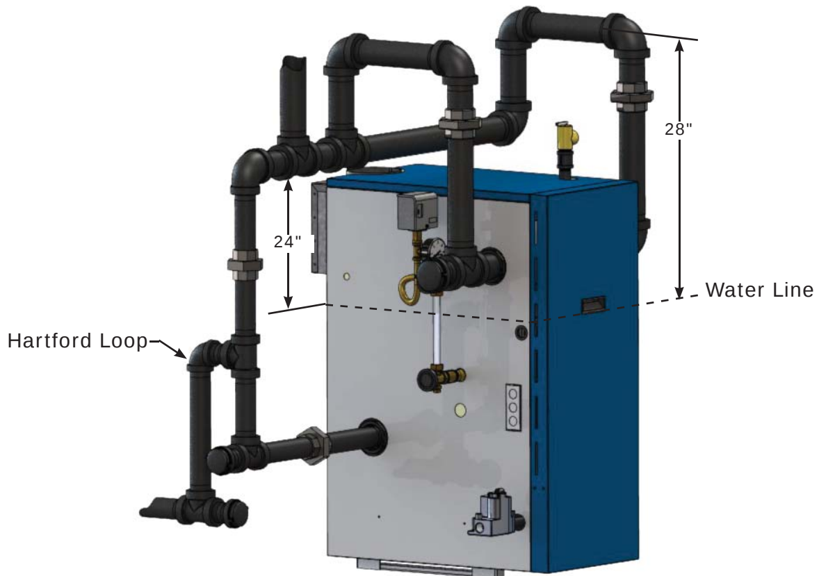
Figure 21 - Drop Header for True Swing Joint
