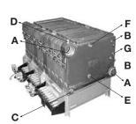
"If opening F is to be used for something other than the Safety Valve or Pressure Relief Valve, or the Safety/Relief Valve is larger than 1", the Safety/Relief Valve must be installed in the Header Piping as near to the boiler as possible.
