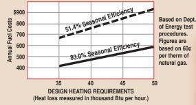
This graph illustrates the difference in annual operating costs between boilers with higher and lower efficiencies. Boilers installed years ago have seasonal efficiencies as low as 50%. So, your savings in fuel dollars with Utica's DV-B boiler can repay its installed cost in a few short years!
